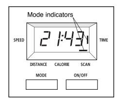
word "SCAN." The speed, time, distance and calorie modes will all be displayed, for five seconds each, in a repeating cycle. A second mode indicator will show which mode is currently displayed.
